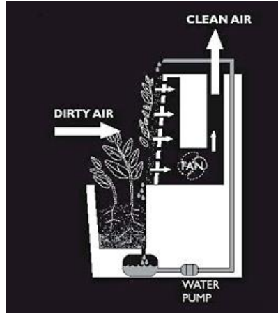
Fig.7 The basic mechanics of a biofiltration wall.
